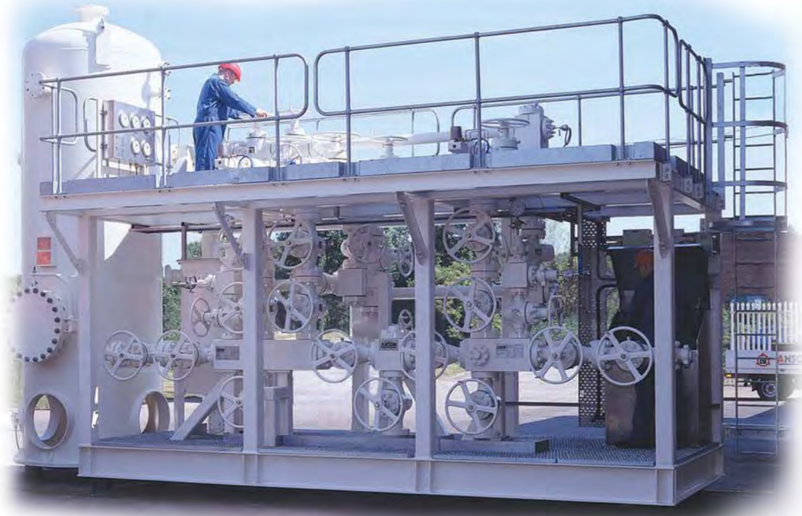
3 1/16" 10,000 psi x 3 1/8" 5000 psi Choke and Kill Manifold
