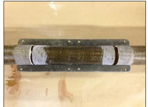
Fig. 12. Damaged areas over 3 inches in length are repaired by replacing the affected pipe with a nipple of appropriate length.
