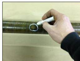
Fig. 1. Impact damage is generally apparent as a whitish discoloration.
