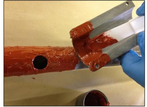
Fig. 6. Apply adhesive to the rim of the hole and to all bonding surfaces.
