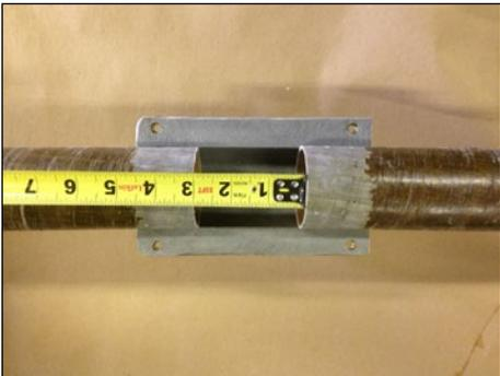
Fig. 10. Damaged areas up to 3 inches in length can be repaired simply by removing the affected pipe and enclosing the gap with a coupling.
