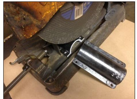
Fig. 15. Cut half-couplings so that all bolt holes are equidistant from the ends. Half-couplings are 7 inches long in 2-inch sizes, and 5½ inches long in 3 and 4-inch sizes.
